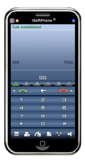
To finish the connection just hit <ESC> or press button. Once the connection is finished then iSoftPhone display's will look like shown below.
